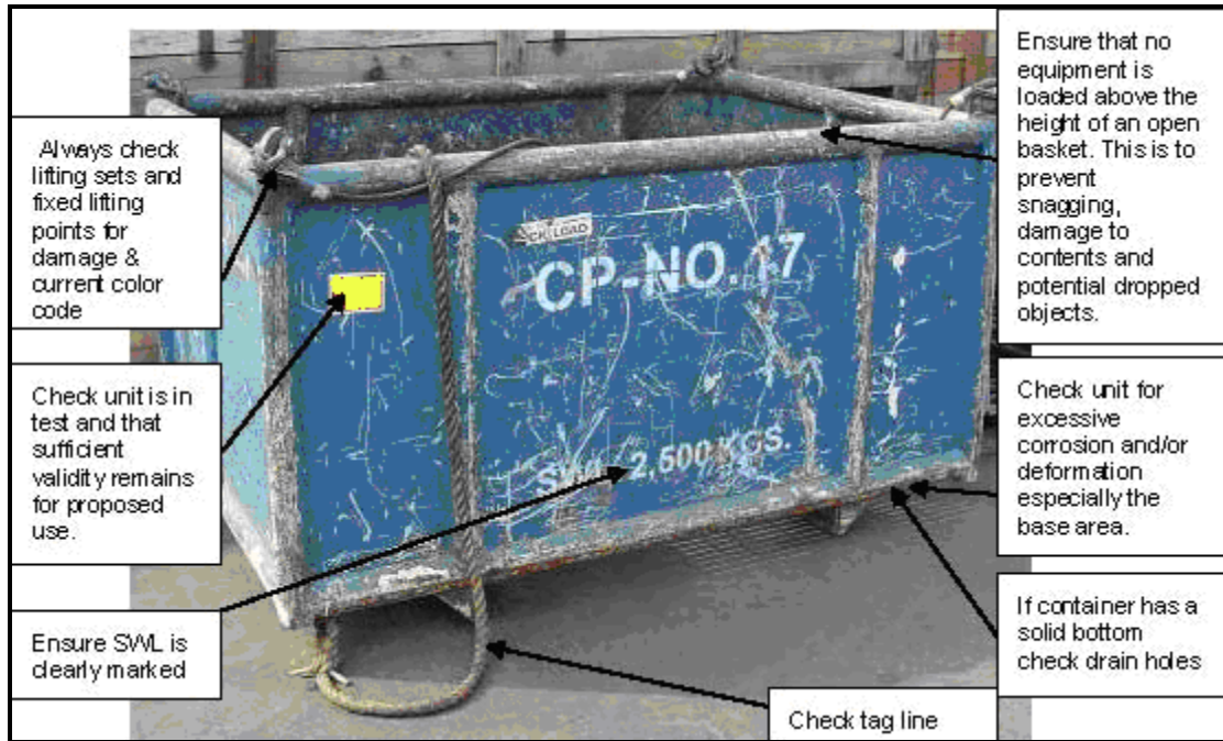
Figure 4. Open Top CCU – Pre-Use Inspection
