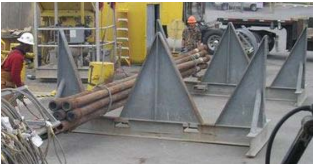
Figure 8. Tubulars Vee-Racking Example
