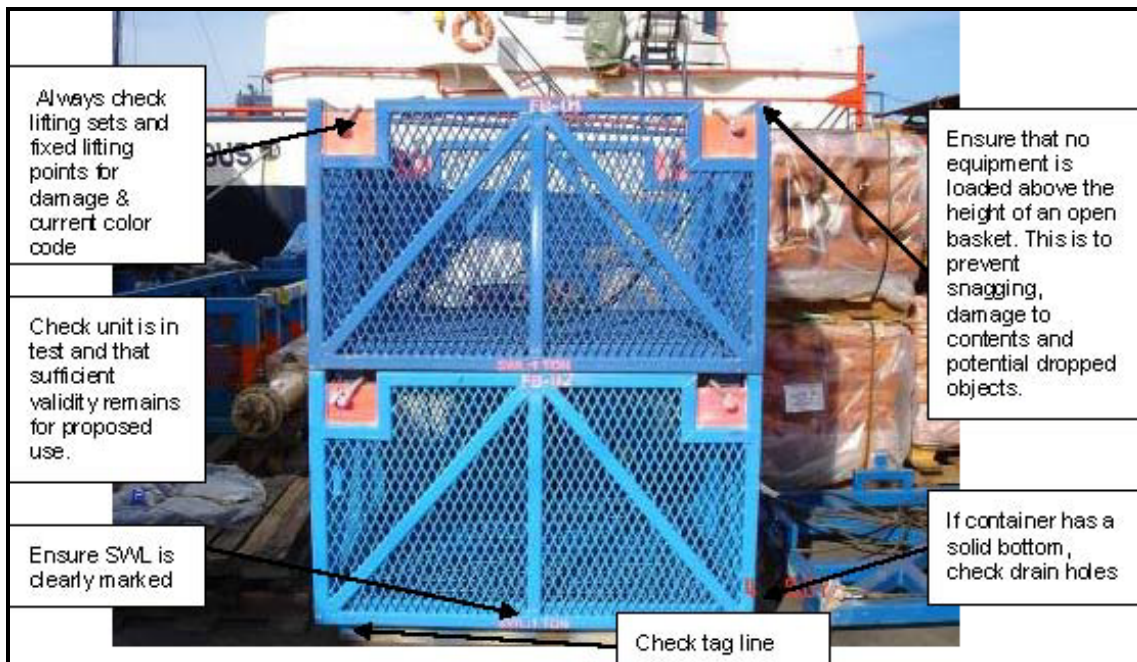
Figure 5. Stackable Baskets – Pre-Use Inspection
